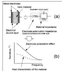
Figure 2. The electrode polarization problem has so far limited the use of permitivitty measurements.
