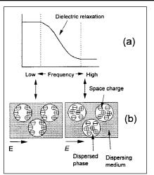
Figure 1. Dielectric dispersion properties provide insight into the nature of colloids: structure, purity and concentration are often related to permittivity.
