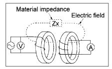
Figure 3. The design of the HP E5050A eliminates electrode polarization, allowing measurement of actual material behavior.
