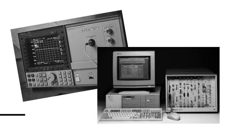
Used as a tunable, bandwidth-variable filter for the HP 75000 Series 90 modular telecom analyzer, the HP 71451B optical spectrum analyzer's monochromator allows access to individual channels of a WDM signal for BERT measurements.
