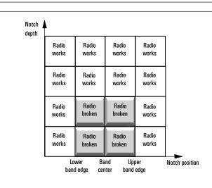
Figure 2. Model of M-curve measurement diagram showing separation of unacceptable and acceptable radio performance.
