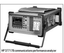
HP 37717B monochrome version providing a budget solution, and a 20-column printer. Both instruments include a 3.5-inch disk drive to ease results retrieval, test firmware upgrades, and analysis.
