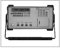
and dispersive fade margin. Its built-in printer provides hardcopy results of both the signature plot and tabular data for comparison with different radios and manufacturer's specifications.
