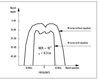
Figure 3. Plot of typical M-curve measurement diagram. The M-curve must always include the threshold BER value and the delay.
