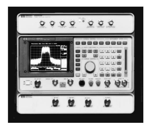
For testing PCS mobiles and base stations with the HP 8920A/B, 8921A, or 8924C, test set
