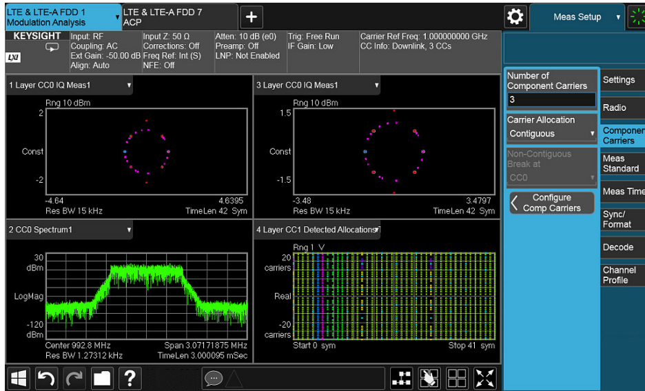
Figure 15. This display of an LTE downlink demodulation result includes the constellations of different signal layers (top) and detected resource allocations (bottom right).
