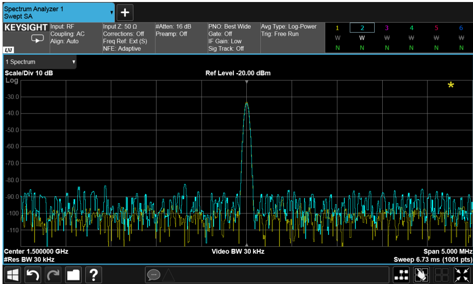
Figure 17. The second-harmonic measurements appear at the same amplitude, indicating that the analyzer's own distortion is not causing an error in the result.
