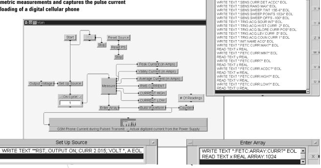
Figure 2. Block flow diagram of the Agilent VEE program, showing program details
