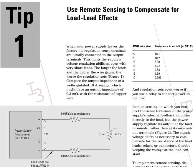
Figure 1: The effects of six feet of AWG 14-gauge leads without remote sensing
