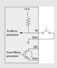
Figure 1. Remote inhibit and discrete fault indicator schematic
