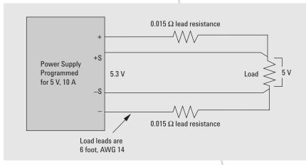
Figure 2: Using remote sensing to correct the lead-load problem
