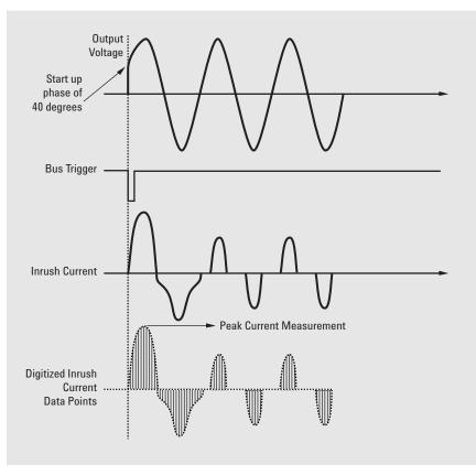
Figure 1: An inrush current measurement at 40° using Agilent 6800 series ac power source/analyzers
