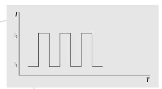
Figure 3: A typical pulse charging waveform created with an electronic load
