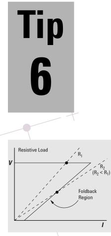
Figure 1: Foldback behavior in constant resistance mode
