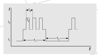
Figure 4: A complex waveform that simulates the energy-saving features in portable, battery-powered products
