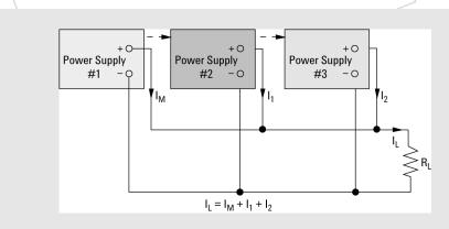
Figure 2: Connecting units in parallel
