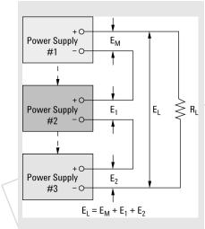
Figure 1: Connecting units in series
