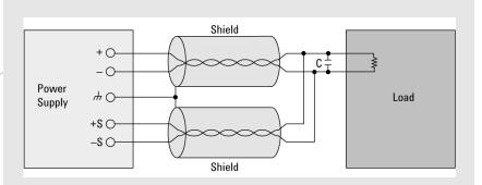
Figure 1: Minimizing radiated pick-up with twisted shield leads for both output and remote sense leads
