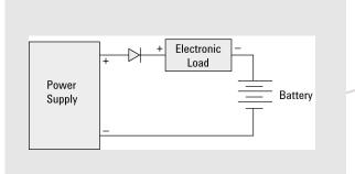
Figure 2: Pulse charging using an electronic load is much faster, while still achieving 90% recharge.
