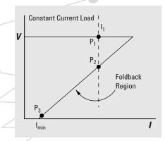
Figure 2: Foldback behavior for constant current load
