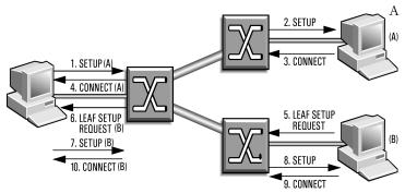
Figure 12: In a root LIJ, leaves join the call by sending a LEAF SETUP REQUEST to the network.
