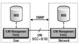
Figure 5: The user and network both contain databases, known as Management Information Bases, which store a variety of information related to the link between the two endpoints.
