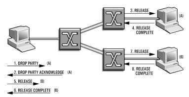
Figure 11: At the end of the P-MP, the root can remove leaves with the DROP PARTY message, or releases the entire call by sending a RELEASE message to the network.
