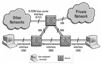
Figure 1: Interaction between the protocols at the user-network interface (UNI) and the network-network interface (NNI).
