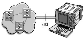
Figure 18: To generate potential non-conforming service requests into a network, an analyzer is connected.
