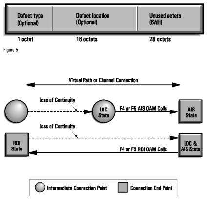
Figure 6: Reporting defects using AIS and RDI cells
