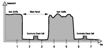
Figure 10: A network node to periodically insert continuity check (CC) OAM cells into the cellstream
