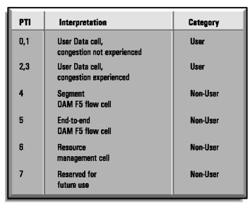
Figure 15: Definition for user cells on the F5 level
