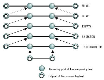
Figure 1: ITU-T considers an ATM network to consist of five flow level
