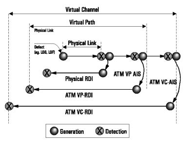
Figure 11: A physical layer alarm eventually causes both path (F4) and channel (F5) OAM RDIs
