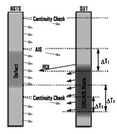
Figure 13: Stops generating AIS or RDI cells after receiving the first continuity check OAM cell
