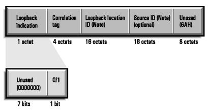
Figure 7: Loopback cells are used determine connectivity at specific points in a network. Note: Values (except for default all 1's) are not subject to standardization and encoding of non-default values is optional.
