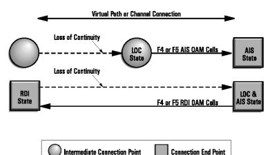
Figure 12: AlS OAM cells should be transmitted on the downstream connection to alert the connection end point  $% \left( {{\left[ {{{\rm{A}}} \right]}_{{\rm{A}}}} \right)$
