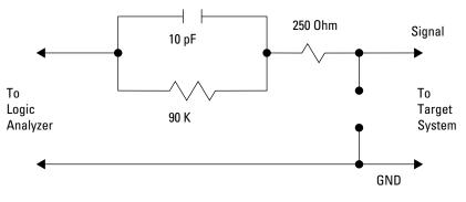
Figure 3. RC Network for Signal Termination
