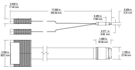
Figure 6. High-Density Termination Adapter Cable Dimension
