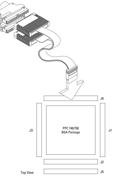
Figure 1. Connector layout for a PPC740/750 BGA target
