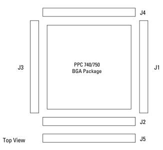
**Figure 4. Mictor Connector Placement**
