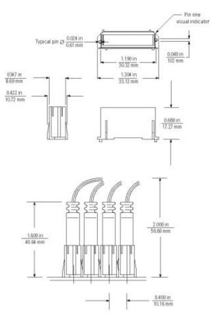
**Figure 7. Support Shroud Dimensions**
