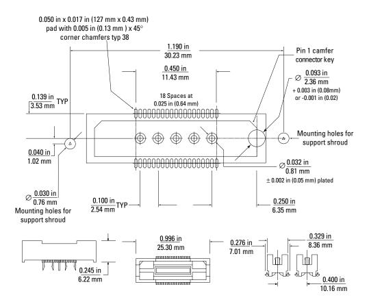
**Figure 5. AMP Mictor Connector Dimension**
