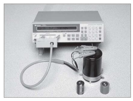
Figure 3. Big Electrodes Electrolytic Capacitors Measurement using the Keysight 16089A
