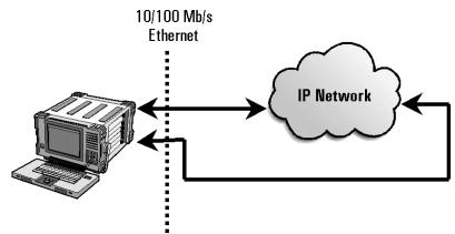
Test configuration #2: Dual-port 10/100 Mb/s Ethernet tester connected to an IP network: This configuration can also be used to test ADSL modems that have Ethernet access ports.
