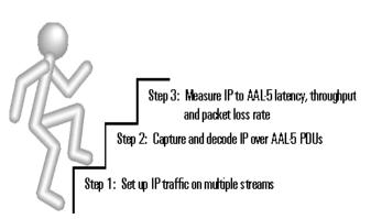
Test methodology for interworking testing of an IP/ATM access device
