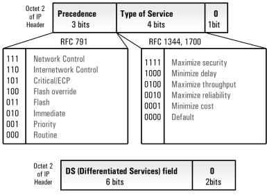
The second octet of the IPv4 header is currently occupied by the TOS and Precedence fields. The IETF may replace them by a 6-bit DS field.
