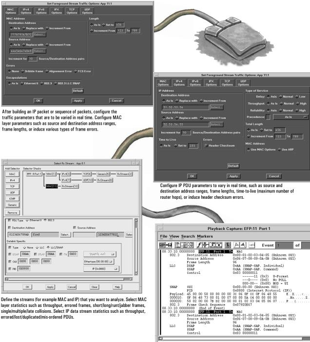
layer statistics such as throughput, errored frames, short/long/runt/jabber frames, single/multiple/late collisions. Select IP data stream statistics such as throughput, errored/lost/duplicated/mis-ordered PDUs.
