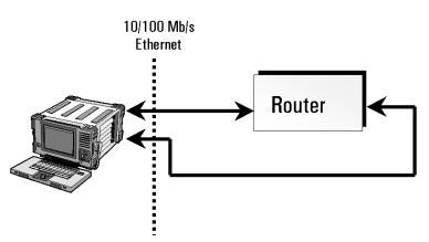
Test configuration #1: Dual-port 10/100 Mb/s Ethernet tester connected to a router.
