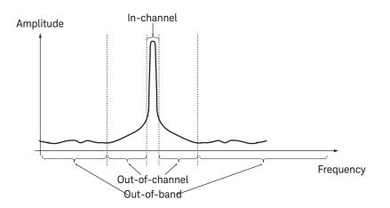
Figure 1. In-channel, out-of-channel, out-of-band measurements
