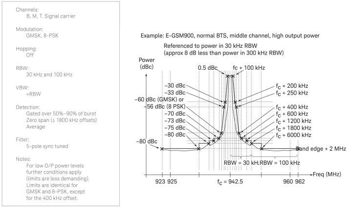
Figure 19. Spectrum due to modulation and wideband noise, normal BTS, limits
