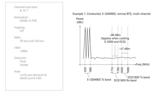
Figure 26. Cross-band spurious, GSM900 into DCS bands, BTS, limits
