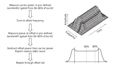
Figure 18. Theory of spectrum due to modulation and wideband noise
