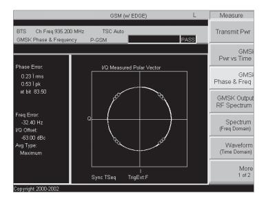
Figure 8. Constellation diagram on the Keysight E4440A PSA series spectrum analyzer showing GMSK modulation
