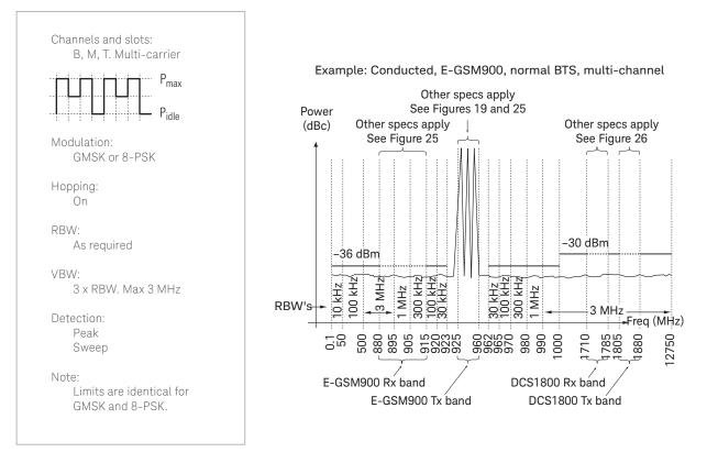
Figure 28. Wideband spurious, BTS, limits
