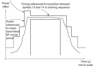
Figure 13. Theory of transmitted RF carrier power versus time
