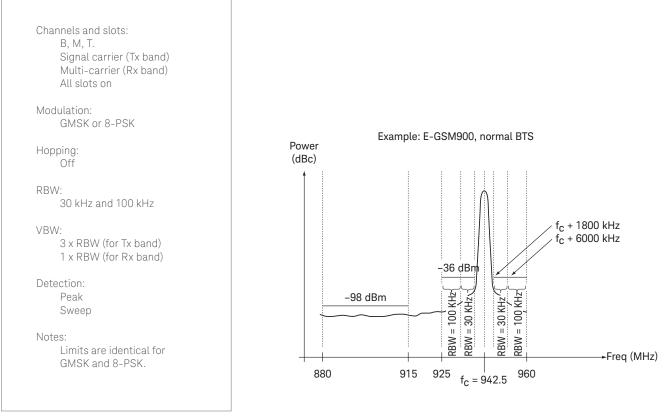
Figure 25. Tx and Rx band spurious, BTS, limits
