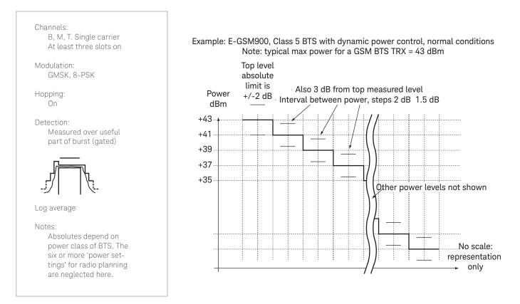
Figure 12. Mean transmitted RF carrier power, BTS, limits
