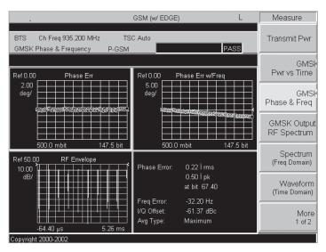
Figure 7. Quad display of the Keysight E4440A PSA series spectrum analyzer showing GMSK modulation metrics graphics of phase error with and without frequency error
