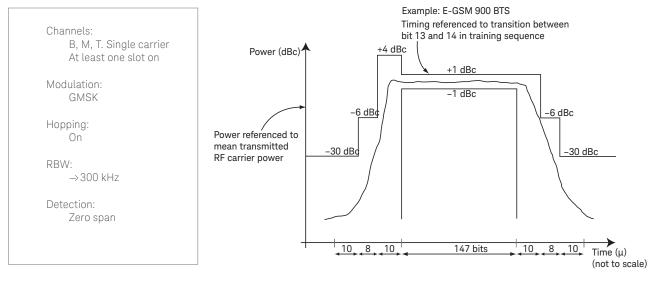
Figure 14. GMSK transmitted RF carrier power versus time, BTS, limits, GMSK
