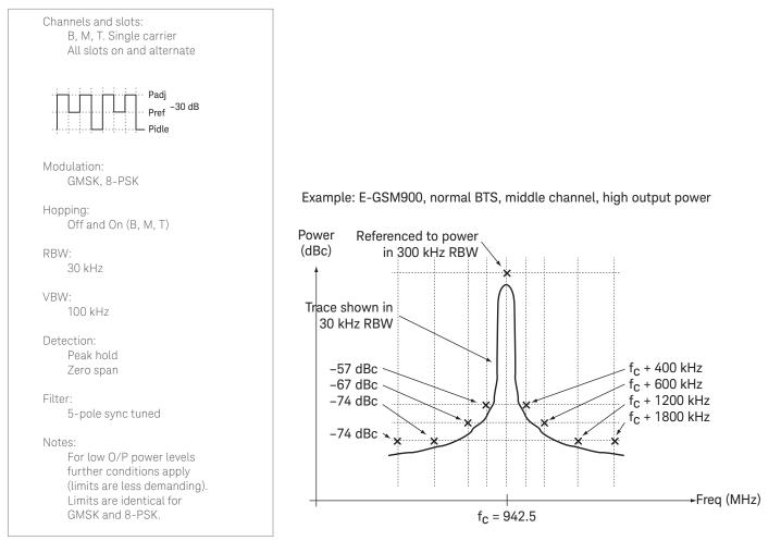
Figure 22. Spectrum due to switching, BTS, limits
