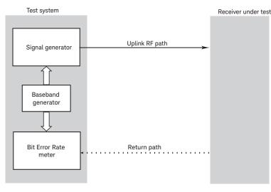
Figure 29. Theory of bit error rate
