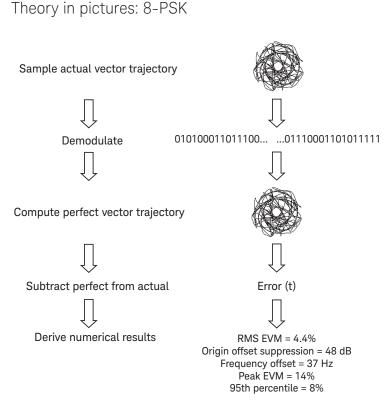
Figure 4. Theory of EVM, origin offset and frequency offset (8-PSK)
