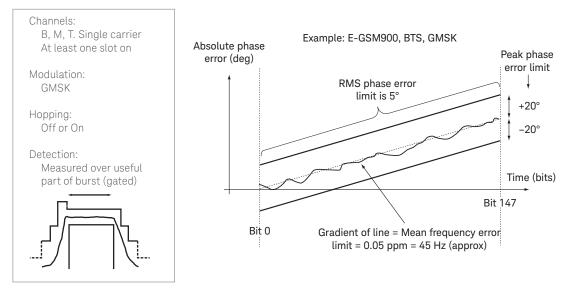
Figure 5. Phase error and mean frequency error, BTS, limits
