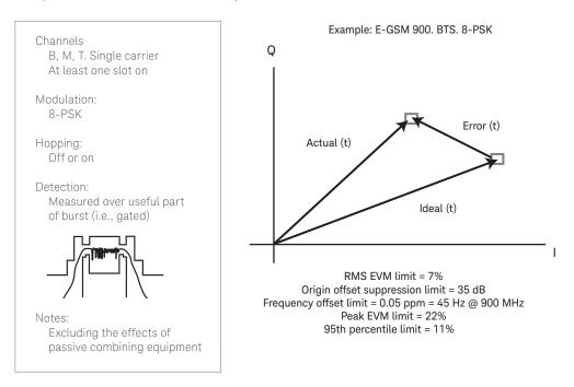
Figure 6. EVM, origin offset and frequency offset, BTS, limits
