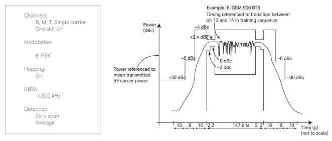
Figure 15. Transmitted RF carrier power versus time, BTS, limits: 8-PSK
