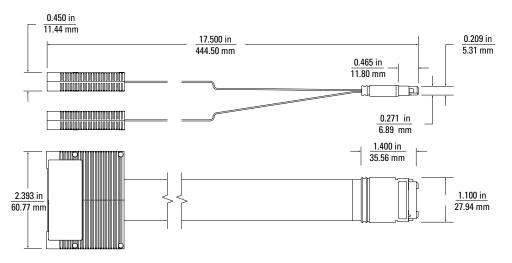
Figure 7. High-Density Termination Adapter Cable Dimensions
