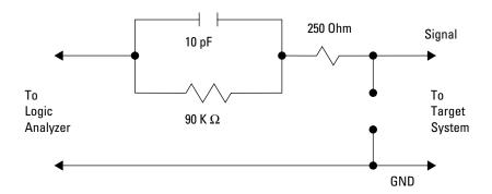
Figure 3. RC Network for Signal Termination
