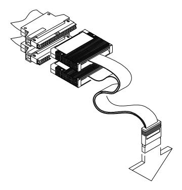
Figure 1. Connector Layout for a Motorola MPC555 BGA Target
