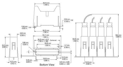
**Figure 6. Support Shroud Dimensions**
