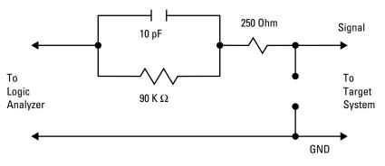
Figure 3. RC Network for Signal Termination
