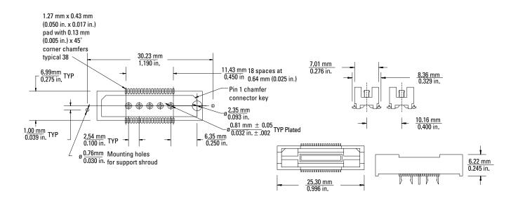
Figure 5. AMP Mictor Connector Dimensions
