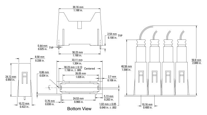
**Figure 6. Support Shroud Dimensions**
