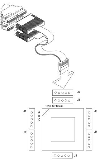
Figure 1. Connector Layout for a Motorola PowerPC 740/750 BGA Target
