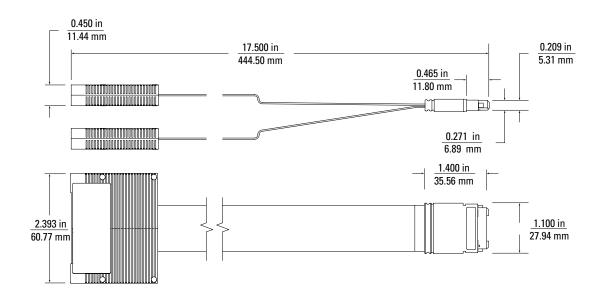
Figure 7. High-Density Termination Adapter Cable Dimensions
