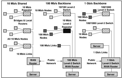
Ethernet LAN Collapsed Backbone Network Evolution
