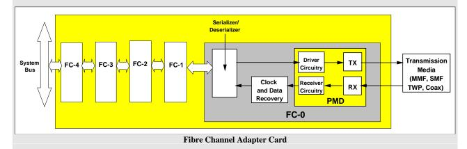
Physical Media Dependent (PMD) products are designed to interface with either copper or multi-mode and single-mode, glass fiber-optic cables. OEMs can design them into various equipment, such as Fibre Channel hubs, switches, or mass storage devices. OEMs can also use some of these products as part of a workstation subassembly
