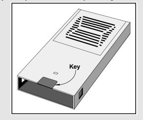
The keying options are based on the specific part of the FDDI LAN that the data communication link fits. The link from a concentrator to a device was defined as a "master-slave" link, while the two redundant rings (described earlier) were called the A ring and B ring. The keying options, shown in the following table, were then defined.
