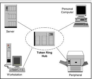
The Token Ring standard specifies a hub-based wiring structure. The hub, which is centrally located, manages the LAN. The Token Ring LAN does not appear to be a ring because the wiring is hidden inside the hub.
