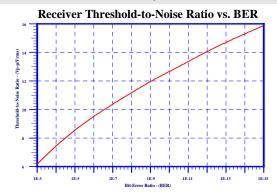
At any fixed temperature the total value of the receiver's random noise plus the host system's noise can be assumed to be a constant. So, the most obvious way to reduce the probability of error is to increase the amplitude of the optical signal applied to the receiver.
