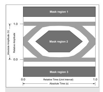
As shown by the preceding diagram, a mask consists of two parts:
