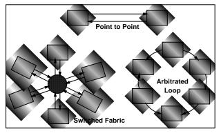
Switched-fabric topologies are used today for clustering multiple devices through a switching fabric. This fabric can be a single switch or a network of interconnected switches, as shown below.
