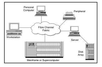
Point-to-point Fibre Channel data communication links are used today for efficient transmission of large blocks of continuous time-sensitive data and are ideally suited for mass storage applications.
