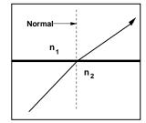
process continues all the way to the end of the fiber. This phenomenon is known as total internal reflection (TIR), a key principle in fiber optics. (The only loss of light is from scattering by foreign matter or by absorption).
