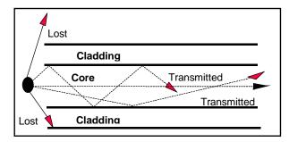
All light rays that enter the fiber at an angle greater than this critical angle,  $\alpha$ , exit through the cladding and are lost. This angle can be calculated based on the value, n, of the core and cladding, and is usually represented as the numerical aperture, NA, a standard specification of any fiber. The NA is defined in the following illustration.
