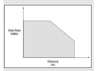
The flat line is where the fiber does not contribute to any limiting effects. The sloping line is where the data rate decreases as the distance increases. Finally, there is a cut-off point, the vertical line, at which the receiver can no longer detect the signal.
