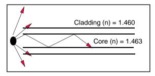
The index of refraction of the core must be larger than that of the cladding for the light to travel through the waveguide:
