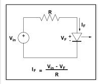
the series resistance. It is the current through the LED that controls the light output.
