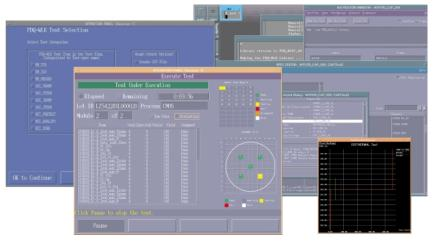
PDQ-WLR test software supports integrated production and development environment reducing cost of ownership. The PDQ-WLR framework with WLR test menu and test execution provide easy-to-use test platform. High accuracy and fast WLR routines actively control critical acceleration for predictive reliability tests.
