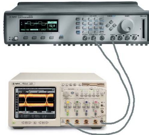
Figure 2. The setup of an Agilent pulse generator and Infiniium oscilloscope.
