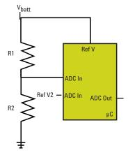
Figure 4: Measuring battery voltage with one reference voltage
