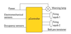
Figure 2: Decentralized airbag system
