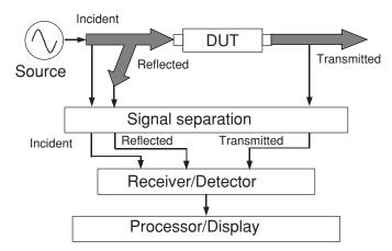
Figure 2. Network analyzer configuration
