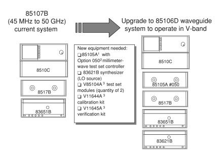
Figure 10. Upgrading an 85107B 50 GHz system to an 85106D waveguide system to operate in V-band (or W-band)
