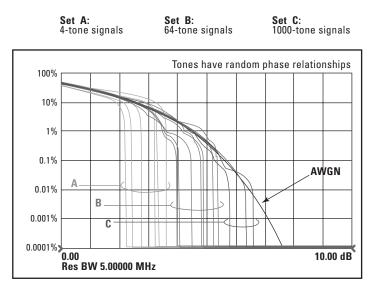
Figure 8: CCDF curves of multiple frequency signals.
