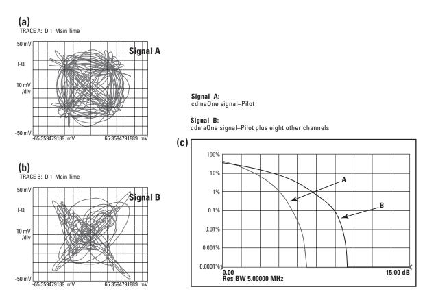
Figure 12: CCDF curves and vector plots of a single-channel cdmaOne signal and a nine-channel cdmaOne signal.
