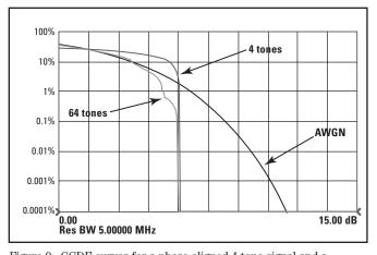
it is possible to generate a signal with fewer tones that is as stressful or sometimes more stressful than a signal with more tones. For instance, *Figure 9* shows that a 4-tone signal with all phases aligned is slightly more stressful than one particular 64-tone signal with random phase relationships.
