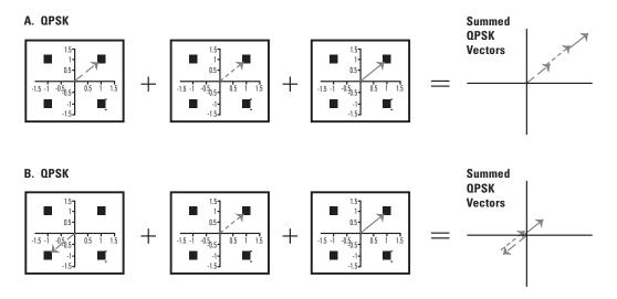
Figure 11: (A) Addition and (B) cancellation of vectors in spread-spectrum systems.
