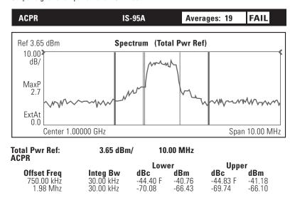
Figure 14: ACPR measurements of amplified signals.
