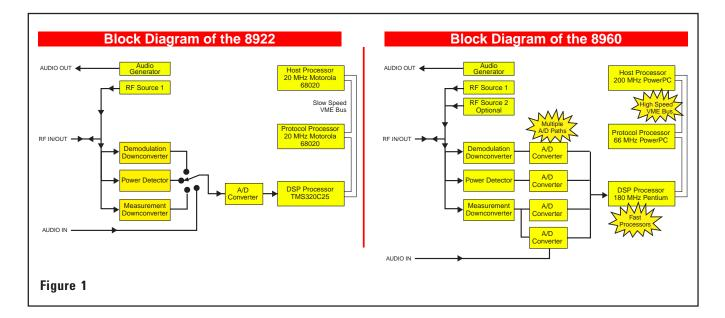
The 8922 has DSP (TMS320C25), and host and protocol processors (20 MHz Motorola 68020). The 8922 has <u>switchable</u> paths for making measurements (measurement downconverter) and maintaining the link (demodulation downconverter).
