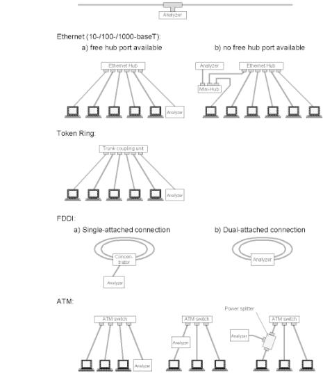
Figure 7: Connecting LAN protocol analyzer systems
