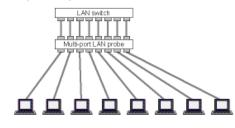
Figure 8: Connection options for protocol analyzer systems in switched LANs
