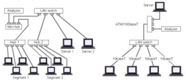
Testing using configurable test ports:
