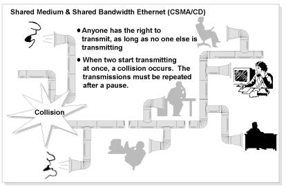
Figure 1: Principles of data communication in local-area networks in the 1980s: CSMA/CD and Ethernet
