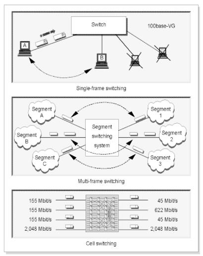
Figure 4: Frame switching and cell switching
