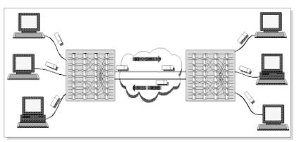
Figure 3: Switching and multiplexing in wide-area data communication
