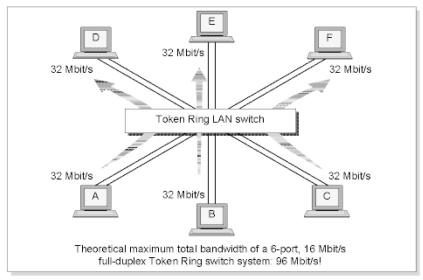
Figure 6: Segment switching and full-duplex Token Ring
