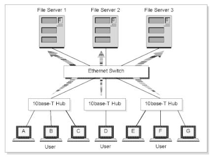
Figure 5: The principle of LAN switching systems
