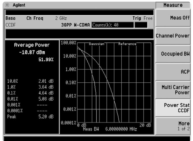
The last part of this exercise involves making power measurements on a four-carrier W-CDMA signal. First the ESG is configured, and then the measurement is made with the PSA.
