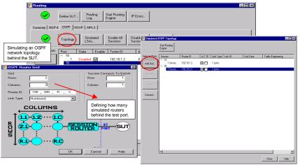
Figure 3: How to add the simulated OSPF topology
