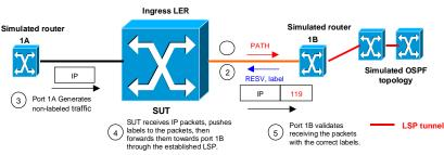
Figure 3: Ingress router test scenario
