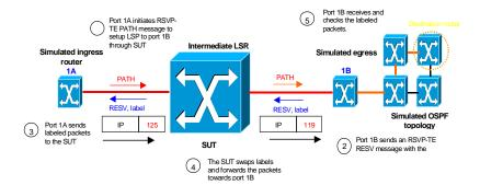
Figure 8: Intermediate router test scenario
