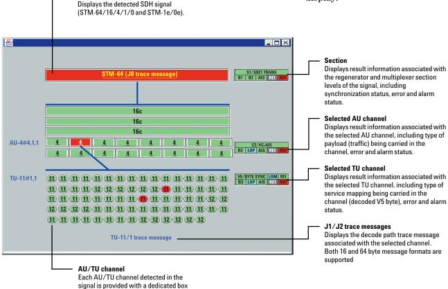
Figure 3: All-channel testing technology
