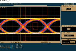
Figure 2. Typical eye diagram
