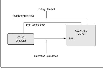
Figure 2. Interconnections for CDMA receiver tests
