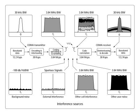
Figure 1. CDMA transmission and reception process
