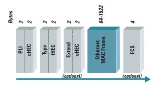
Figure 2. Ethernet in frame-mapped GFP.
