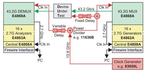
Figure 2: ParBERT 81250 43.2 Gb/s setup for device under test (DUT) characterization. Bit error ratio (BER) measurements with variable sampling delay are realized by a mechanical variable delay line. The fixed delay must be adjusted only once to avoid DUT setup-and-hold time violations.
