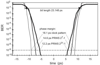
Figure 5: Performance of a ParBERT 43G MUX/DEMUX setup evaluated from bit error ratio (BER) vs. delay (bath tub) plots at 43.2 Gb/s, automatically measured with a setup as shown in Figure 4. The phase margin values, which are evaluated exemplarily at a BER threshold of  $10^{-9}$ , are not corrected by the additionally inserted random jitter from the 10.8G system.
