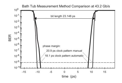
Figure 6: Comparison of bath tub plots at 43.2 Gb/s measured with a manual (see Figure 3) and an automatic (see Figure 4) ParBERT 81250 setup. Phase margin values are evaluated exemplarily at a BER threshold of  $10^{-9}$ . The deviation in the phase margins results from inserted random jitter from the 10.8G system
