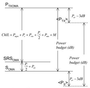
Figure 2. The 10Gigabit Ethernet power budget
