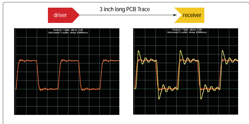
Figure 1. A signal as it emerges from the driver chip (left) is distorted by multiple reflections from impedance discontinuities at both ends (right).
