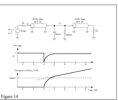
remaining component of the integral is due to the shunt capacitance.
