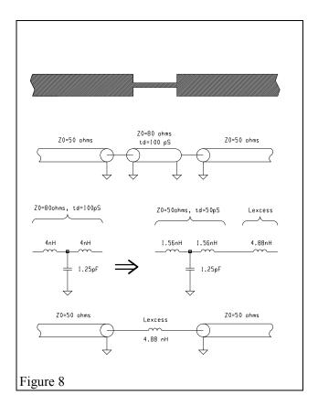
In this case, the portion of the total inductance that balances the total capacitance is
