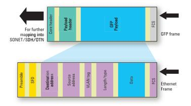
the client bit stream, the GFP source adaptation process deletes the gaps between the packets, known as the Inter Packet Gaps (IPGs). Ethernet MAC is then forwarded for further encapsulation into the GFP frame. On the sink side, the sink adaptation process restores the IPGs, and Ethernet MAC is then forwarded to the client layer for further processing.
