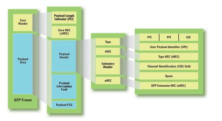
Figure 2. The fields used to describe the GFP frame
