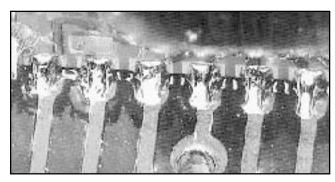
Figure 7.14 Good Solder Joint.
