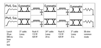
Figure 18. Differential Hspice schematic shows piecewise linear source, lossy transmission line segments, lumped LC flush connector and termination.
