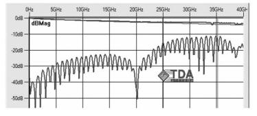
Figure 20. Simulated insertion loss (top) and return loss (bottom) for 30" backplane cable assembly with 112femtoFarad connector.
