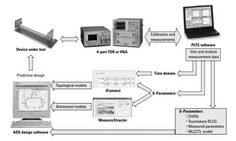
Figure 3. Many different methods exist today for model extraction, but measurement-based model extraction is a relatively new process yielding insight into high frequency effects.
