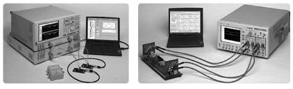
Figure 4. High-speed differential interconnects need to be characterized with a 4-port measurement system, whether it be a 4-port VNA (left) or 4-channel TDR (right).
