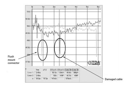
Figure 16. Impedance discontinuities from two different physical structures can look very similar. However, the intuitive nature of TDR's helps discriminate between and break in the cable and the flush mount connector.
