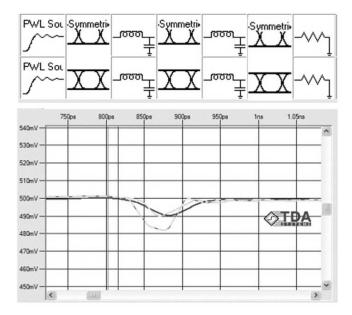
Figure 19. Superimposing the differential schematic of the cable assembly with the impedance profile indicates a connector shunt loss that causes a 5 ps degradation.
