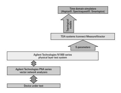
Figure 12. The first model extraction method used in this experiment used measurements from a VNA, then exported the 4-port S-parameters from PLTS directly into MeasureXtractor. A topological model was then exported from MeasureXtractor into Hspice.
