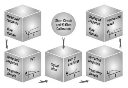
Figure 8. Time domain normalization is an error correction technique that resides in firmware inside the TDR oscilloscope. This technique utilizes the Bracewell Transform developed at Stanford University and removes test fixture error by performing frequency domain math functions.
