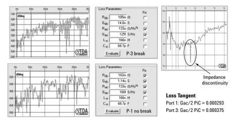
Figure 15. Backplane cable assembly lossy models shows loss tangent with impedance discontinuity due to cable defect on one side of differential pair.
