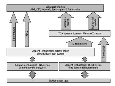
Figure 11. An overview of the many ways to develop models for digital interconnects.
