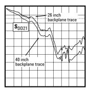
Figure 6. Example of typical 4-port analysis using both time and frequency domain data. Note: this is just an example from a 3 Gb/s backplane, not from the design case study device.
