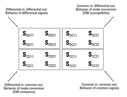
Figure 5. The sixteen S-parameters that are obtained by fully characterizing a differential interconnect can be categorized into 4 stimulus/response quadrants: differential in/differential out, common in/common out, common in/differential out and differential in/common out.
