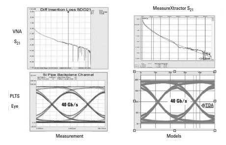
Figure 13. Correlation of input differential insertion loss ( $S_{DD21}$ ) and 40 Gb/s eye diagram was very good between measurement and simulation.
