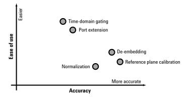
Figure 7. Various mathematical computations and error correction techniques can be made to enhance measurement accuracy. Usually, ease of use and degree of accuracy are inversely proportional to each other.
