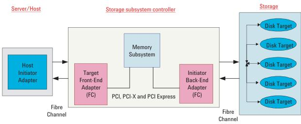
Figure 1. Host Controller - Storage Model
