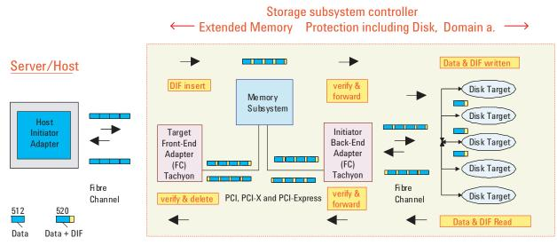
Figure 2. Host Controller - Storage with DIF
