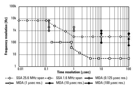
Figure 7. Time and frequency resolution comparison of the signal source analyzer verses a modulation domain analyzer
