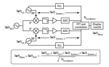
Figure 5. Cross-correlation implementation on the E5052A signal source analyzer
