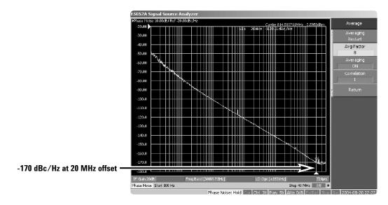
Figure 3. Free-running VCO measurement with high sensitivity of far-out offset frequencies
