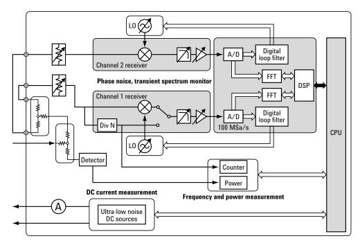
Figure 4. Agilent E5052A signal source analyzer block diagram
