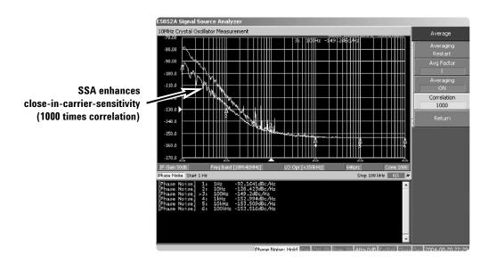
Figure2. Low phase noise crystal oscillator measurement using the cross-correlation technique
