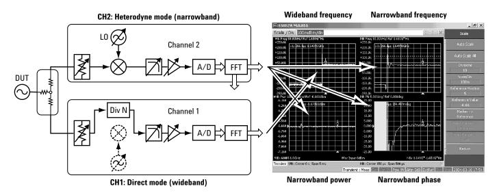
Figure 6. Block diagram of signal source analyzer's dual channel measurement
