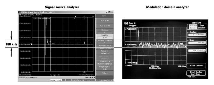
Figure 8. Comparison of SSA and MDA transient measurements
