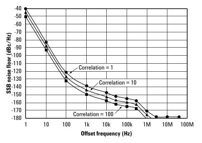
Figure 1. E5052A's Internal SSB phase noise (carrier= 1 GHz, correlation= 1, 10, 100)
