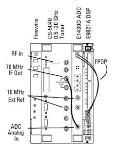
500 MHz - 20 GHz µWave VXI Tuner for Coverage to Greater than 60 GHz
