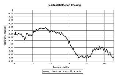
Figure 3. Residual reflection tracking compared
