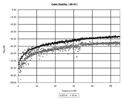
Figure 6. Vector magnitude change caused by a 1-inch movement at end of cable
