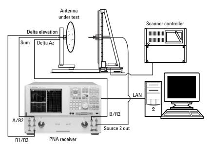
Figure 1: Typical near-field antenna measurement configuration using a PNA with option 014.
