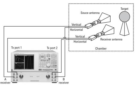
Figure 2: Typical RCS measurement configuration for measuring the full polarization matrix, using the PNA receiver.
