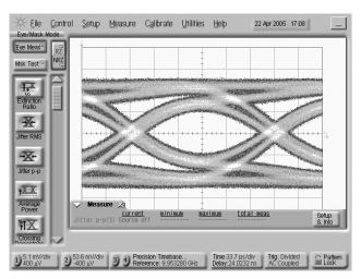
Figure 13: Waveform for ISI on backplane
