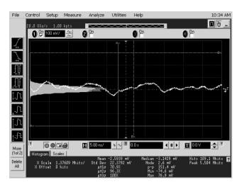
Figure 9: Histogram of voltage signal
