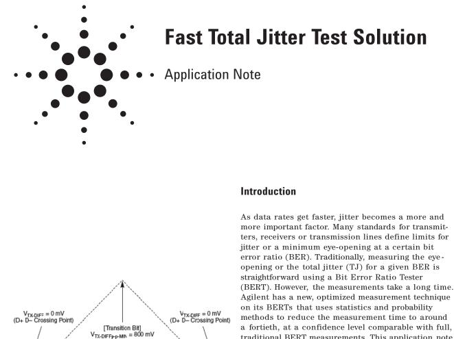
Agilent has a new, optimized measurement technique on its BERTs that uses statistics and probability methods to reduce the measurement time to around a fortieth, at a confidence level comparable with full, traditional BERT measurements. This application note compares the results, measurement times and other considerations for the new Agilent Fast Total Jitter measurement with the traditional measurement, and with the functions available on BERTs and 'scopes to extrapolate eye-opening or TJ.
