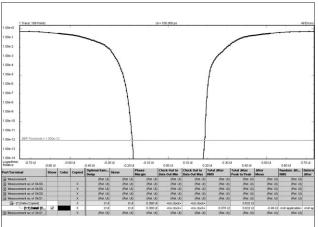
Figure 11: BERTScan 10<sup>13</sup> for bounded gaussian RJ
