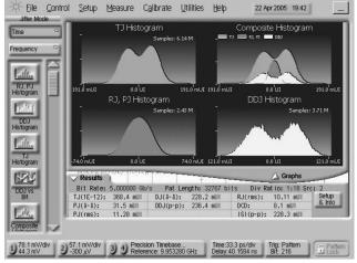
Figure 16: Waveform for ISI on backplane
