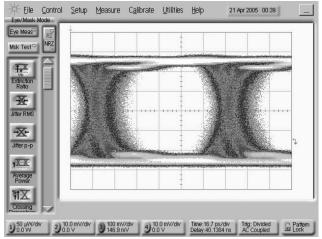
Figure 12: Waveform for bounded gaussian RJ
