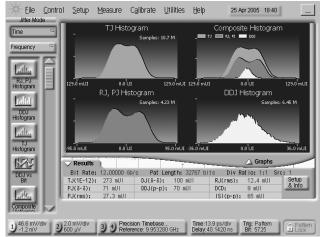
Figure 8: Jitter Analysis on DCA-j for SJ
