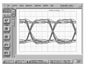
Figure 21: Waveform for a PCI Express video card
