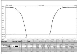
Figure 19: BERTScan 10<sup>13</sup> for an optical transceiver
