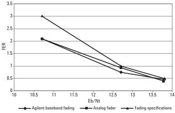
Graph 2: US PCS channel 1175, 30 Km/hr – 1 path – eighth data rate fading comparison
