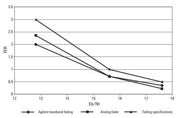
Graph 10: US Cellular channel 1013 – 30  $\rm Km/hr$  – 1 path –eighth data rate fading comparison
