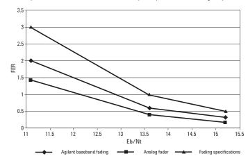
Graph 7: US Cellular channel 384 – 30  $\rm Km/hr$  – 1 path – full data rate fading comparison
