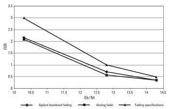
Graph 8: US Cellular channel 384 – 30  $\rm Km/hr$  – 1 path – half data rate fading comparison
