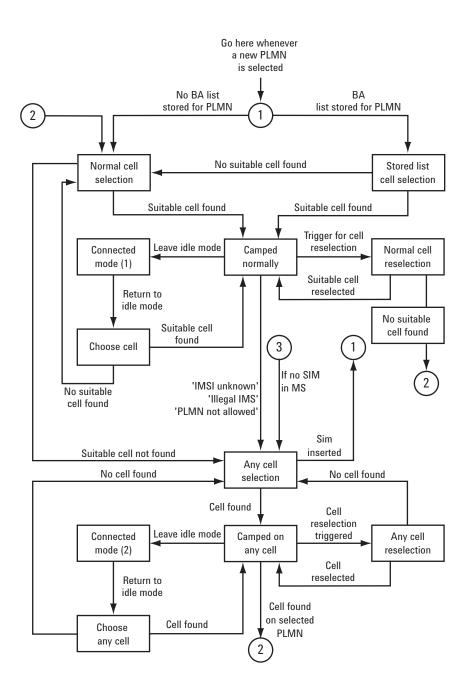
Figure 1. GSM/GPRS/EGPRS cell selection process.
