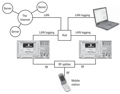
Figure 4. Two-cell test system setup diagram.
