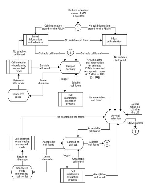
Figure 2 shows the cell selection process and the many states that the W-CDMA/HSDPA MS transitions between as defined in 3GPP TS 25.304 version 3.e.0 Release 99.
