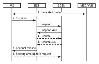
Figure 3. Suspend and resume procedure for intra-SGSN.
