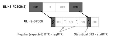
Figure 6. A statDTX is an unexpected DTX response.
