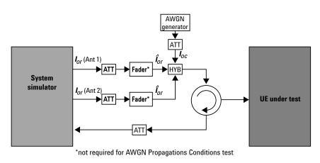
Figure 18. Connection setup for all HSDPA performance requirement tests for open-loop and closed-loop diversity (ref: 3GPP TS 34.121 figure A.19).
