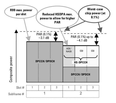
Figure 1. HS-DPCCH increases uplink peak-to-average power ratio (PAR).
