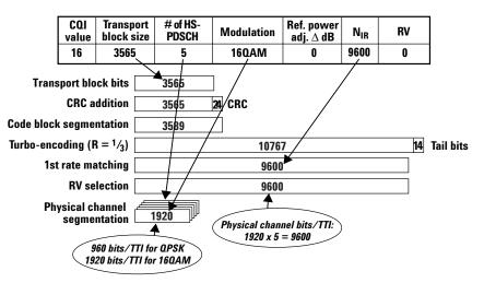
Figure 26. The downlink HS-DSCH configuration for the Reporting of CQI tests is based on a CQI value linked to specific parameters.
