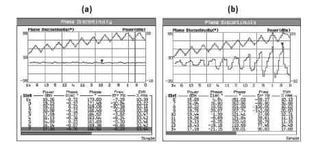
Figure 14. Measuring phase discontinuity can provide an indication of susceptibility to HS-DPCCH power steps. (a) UE with very stable output phase versus 1 dB power steps, and (b) UE with very poor output phase versus 1 dB power steps.
