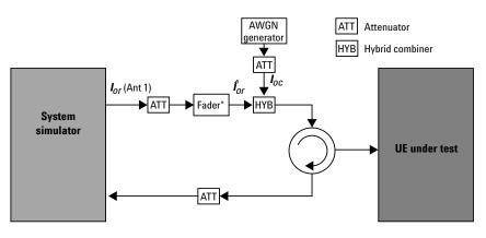
Figure 17. Connection setup for all HSDPA performance requirements tests for single-link performance (ref: 3GPP TS 34.121 figure A.16).
