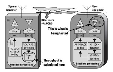
Figure 15. Maximum Input Level for HS-PDSCH Reception with 160AM verifies UE ability to demodulate a 160AM downlink channel.
