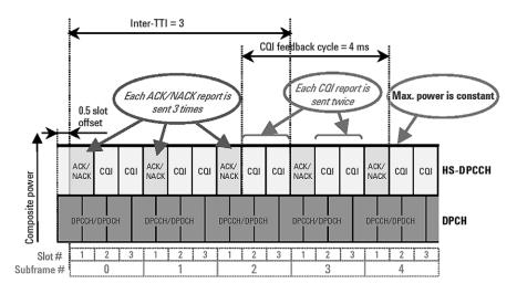
Figure 9. Generic uplink test signal is used for the maximum output power, SEM, and ACLR tests.
