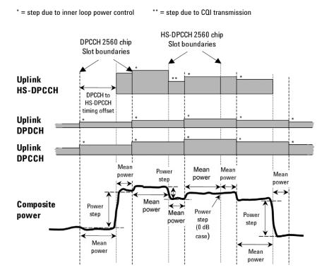
Figure 2. Transmit power template during HS-DPCCH transmission (ref: 3GPP TS 25.101 figure 6.6).
