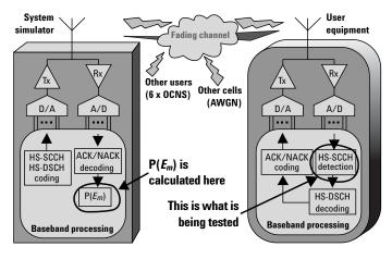
Figure 30. The HS-SCCH Detection Performance test verifies that HS-SCCH detection in the UE is working properly.
