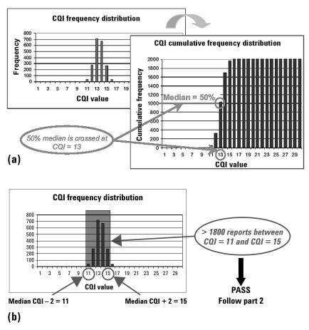
Figure 27. The CQI frequency distribution and CQI cumulative frequency distribution are used to determine (a) the median and (b) the variance of the CQI reports.
