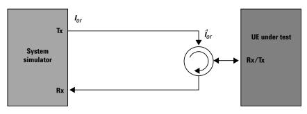
Figure 16. Connection setup for Maximum Input Level for HS-PDSCH Reception with 160AM is identical to that of W-CDMA receiver tests (ref: 3GPP TS 34.121 figure A.3).
