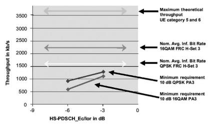
Figure 23. This example shows the relationship among maximum theoretical throughput, nominal average information bit rate, and minimum t-put R requirements for a UE category (based on 3GPP TS 34.121 tables 9.2.1.4 and 9.2.1.6).
