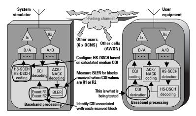
Figure 28. Reporting of CQI under Fading Propagation Conditions tests the accuracy of CQI reporting under multi-path propagation conditions.
