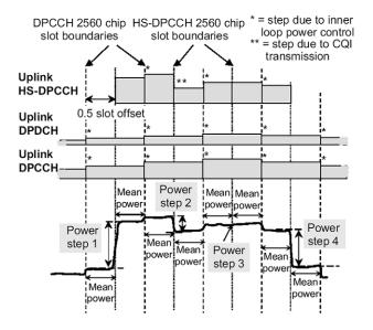
Figure 11. Transmit power template during transmit on/off power – HS-DPCCH measurements (ref: 3GPP TS 34.121 figure 5.7A.2).
