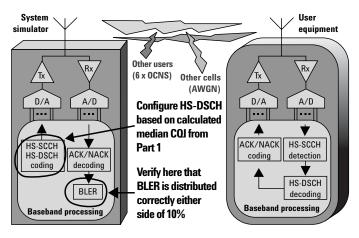
Figure 25. The second part of the Reporting of CQI under AWGN Propagation Conditions test measures BLER distribution for HS-DSCH configured around the median CQI.
