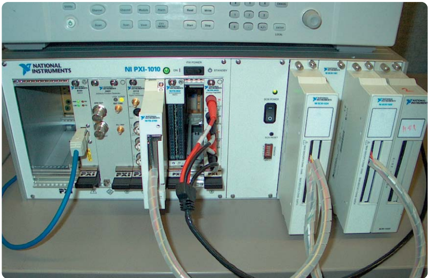
Figure 4. An NI PXI/SCXI cage with an NI MXI-3 interface. PXI cardcages typically require the use of either embedded PCs or external PCs with controller cards installed in them.
