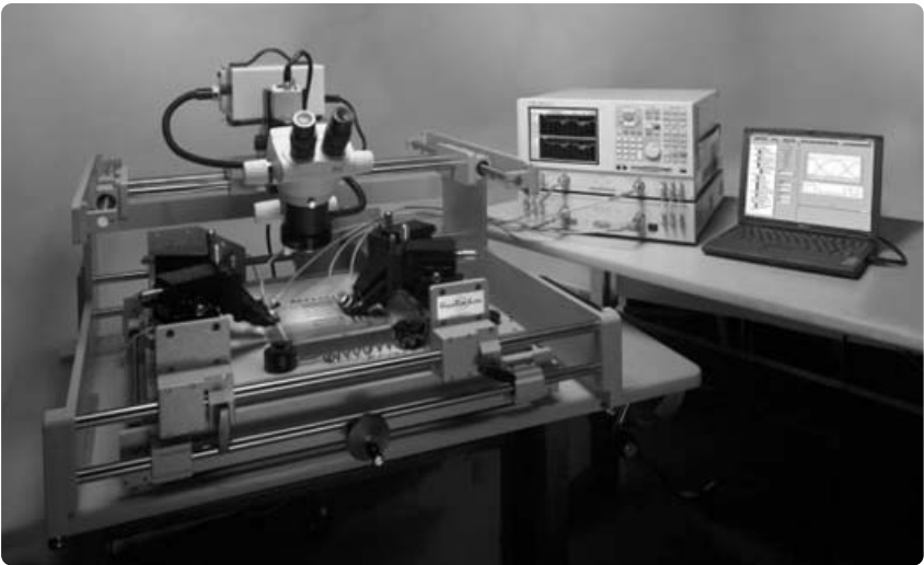
Figure 12. High precision/high frequency probe station (GigaTest probe station)
