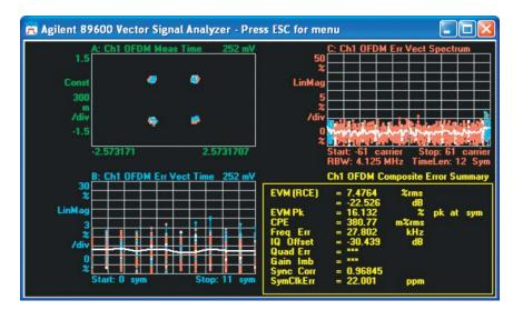
Figure 1. Option BHB MB-OFDM ultra-wideband modulation analysis offers detailed error analysis down to the individual carrier (Trace C, upper right) or individual symbol (Trace B, lower left). For an overall view, composite errors are shown in the table (Trace D, lower right).
