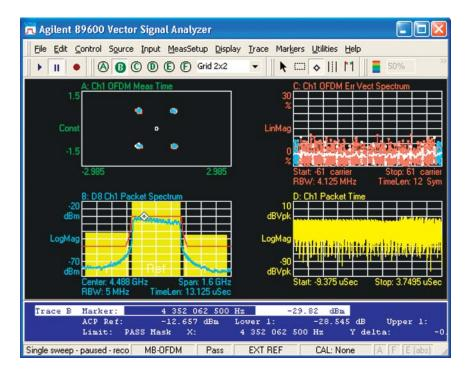
Figure 2. Use the powerful ACP calculation markers and limit lines on the packet spectrum displays to perform important spectral measurements.
