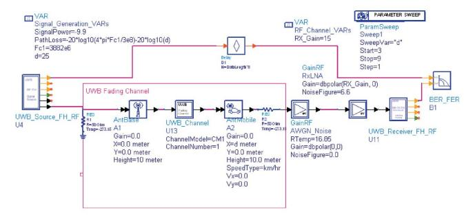
Figure 5. Schematic of UWB MB-OFDM BER measurement with fading channel
