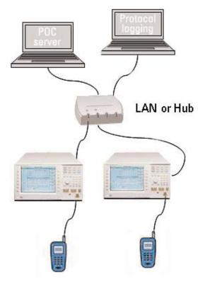
Figure 2. PoC test setup
