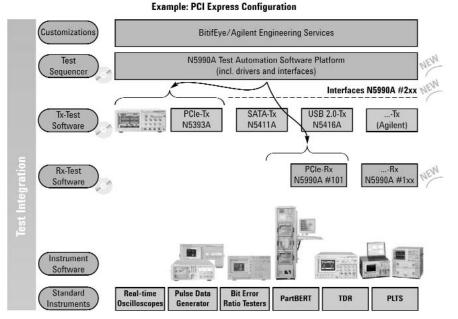
Figure 2: N5990A test platform.
