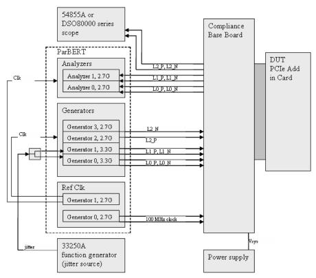
Figure 3: ParBERT configuration for multi-lane PCI Express add-in card receiver physical layer compliance tests.
