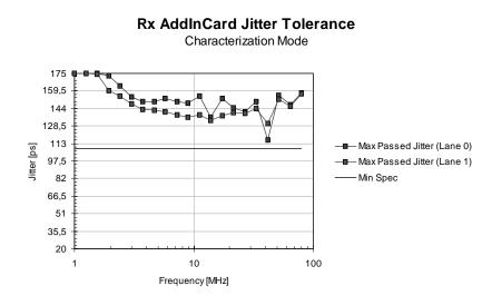
Figure 8: Dual-lane PCI Express receiver jitter tolerance test results.
